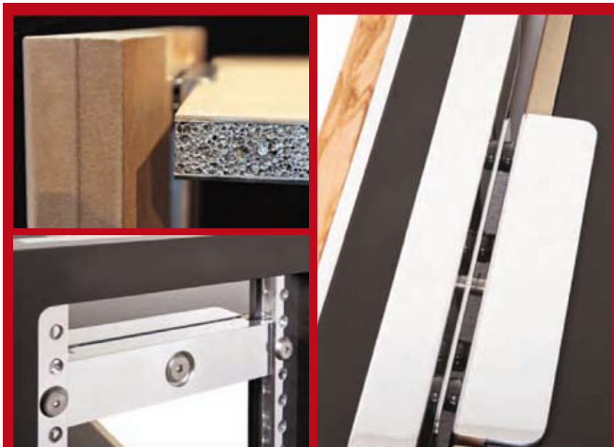
The load-bearing element used for the levels is an aluminium foam laminated with aluminium and MDF (top left). Strong bolts hold them at the desired height in the side panels (bottom left), where – typical for Finite Elemente – ceramic balls create defined transfer points. These can be seen within the gap (right).
