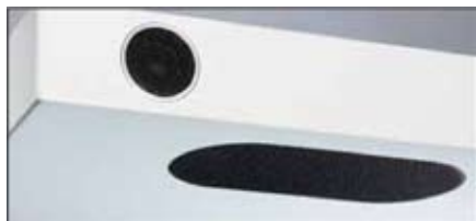
The small tweeters on the front are backed up by two bass/midrange drivers on the underside of the board (above).
