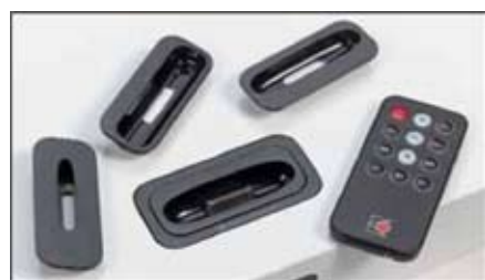
Included are a mini remote control (right) and the standard set of different iPod adapters.
